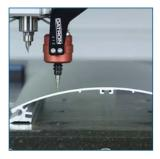
The entire probe assembly is a plug and play component and can be installed in the field. This typically can be done by the customer if desired. Machines are pre-wired for the probe option. Scheduled maintenance is minimal for the probe. An oil reservoir needs to be monitored monthly which is used for a dampening effect on the arm motion.
